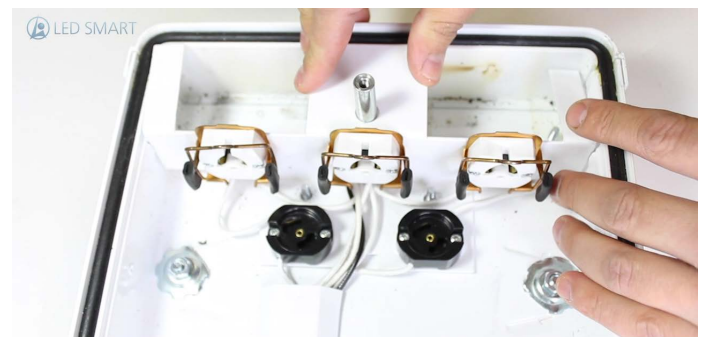
14. Put the lamp holder support bracket back into place
