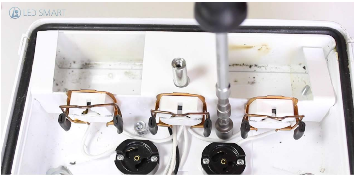
15. Put nuts back into place on the lamp holder support bracket
